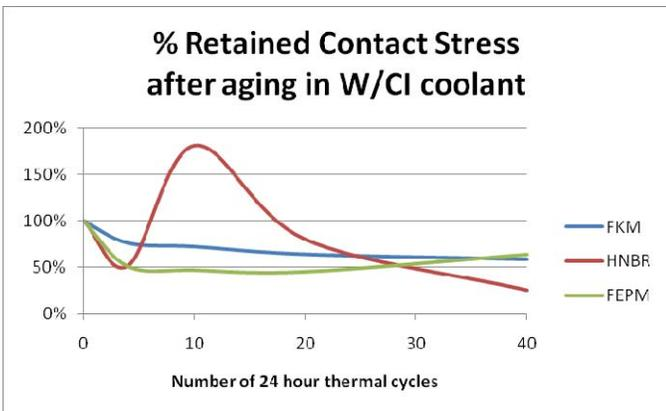
**Figure 32 – Retained Contact Stress in W/CI**
