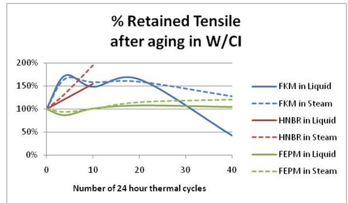
**Fig 7 – D1414 Retained Tensile after aging in W/CI**
