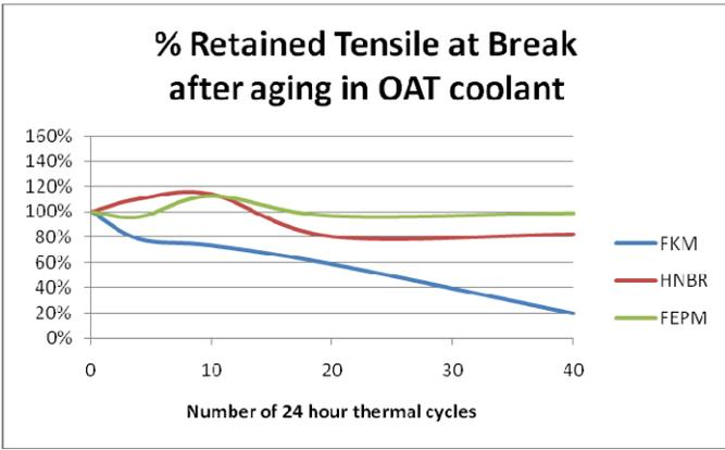
Fig 8 – D412 Retained Tensile in OAT
