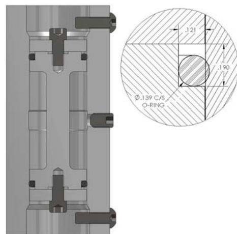
Figure 1 – SK2264, radial deflection of o-rings
