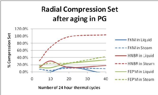
**Fig 21 – Radial Compression Set in PG**
