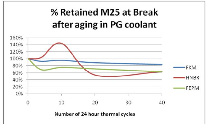
Fig 18 – D412 Retained M25 in PG
