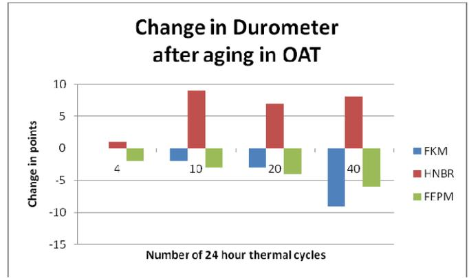
Fig 29 – Change in Hardness after aging in OAT
