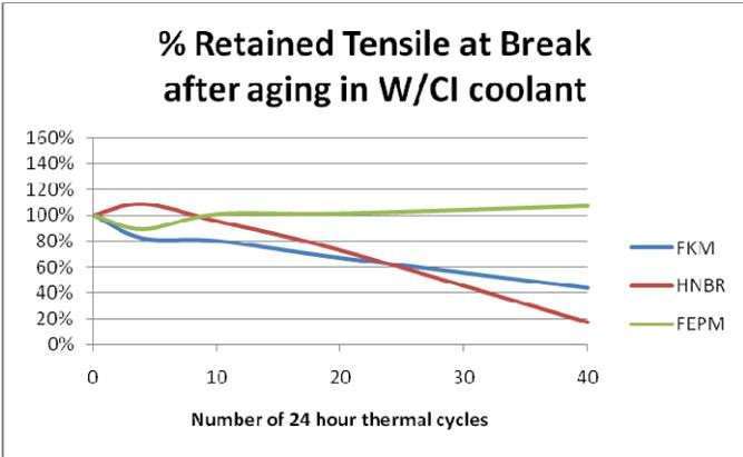
Fig 10 – D412 Retained Tensile in W/CI
