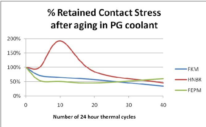
**Figure 33 – Retained Contact Stress in PG**
