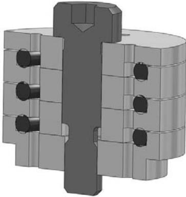
**Figure 2 – SK2451, axial deflection of o-rings**
