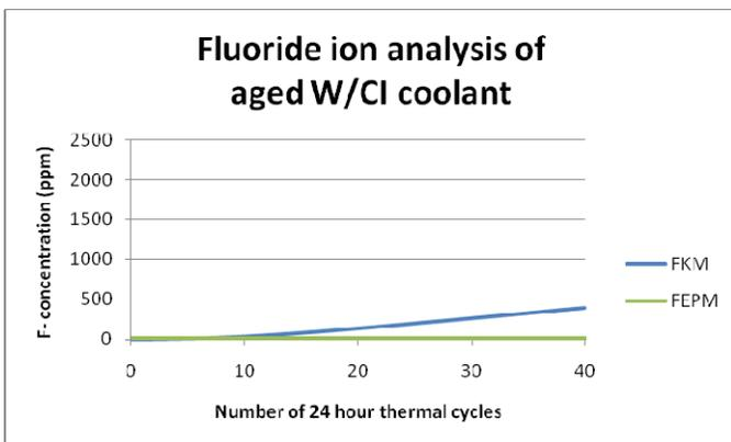
Figure 38 – Fluoride Ion of W/CI Coolant
