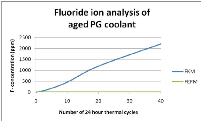
Figure 37 – Fluoride Ion of PG Coolant
