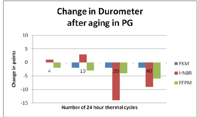
Fig 30 – Change in Hardness after aging in PG
