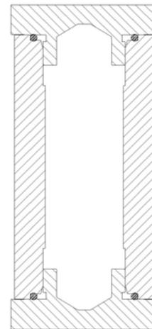
**Figure 4 – SK2451-V Gray Iron aging vessel**
