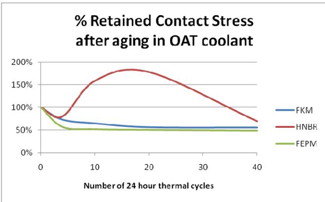
**Figure 32 – Retained Contact Stress in OAT**
