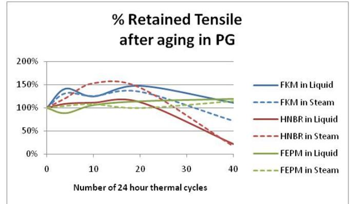
**Fig 6 – D1414 Retained Tensile after aging in PG**
