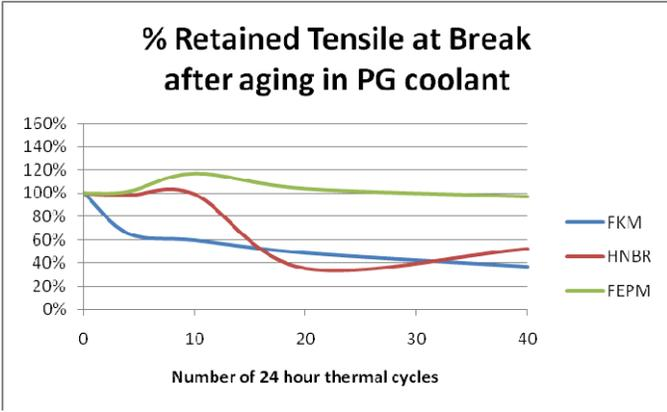
Fig 9 – D412 Retained Tensile in PG
