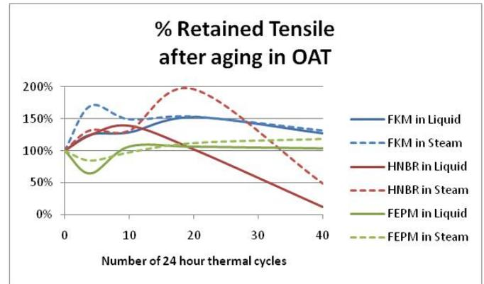
**Fig 5 – D1414 Retained Tensile after aging in OAT**
