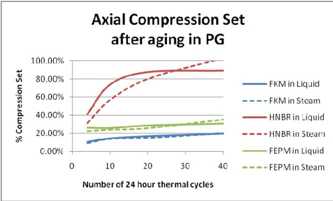
Fig 27 – Axial Compression Set in PG
